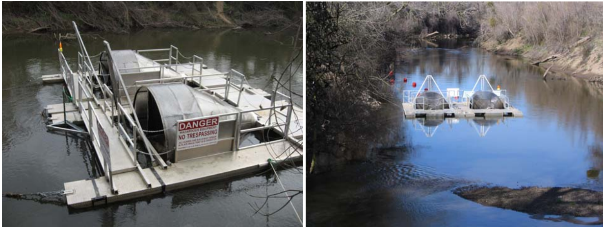
Figure 3. The north and south rotary screw traps positioned side-by-side (left), and upstream view of RSTs at Caswell (right) showing safety buoys and exposed gravel bar.
