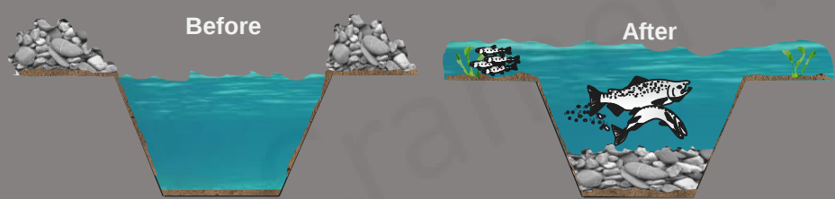
Adding mine tailing into the channel to restore spawning habitat
